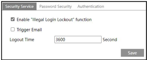
In order to prevent against malicious password unlocking, “Illegal Login Lockout” function can be enabled here. If this function is enabled, login failure after trying five times will make the login interface locked. The camera can be logged in again after a half hour or after the camera reboots.
