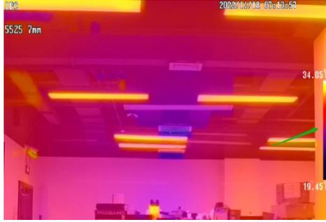
The current minimum and maximum temperature of the scene will display. The minimum temperature shows at the bottom of the bar; the maximum temperature shows on the top of the bar.
