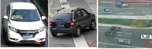
4. Make sure cameras can view objects for at least 2 seconds in the detected area for accurate detection.
