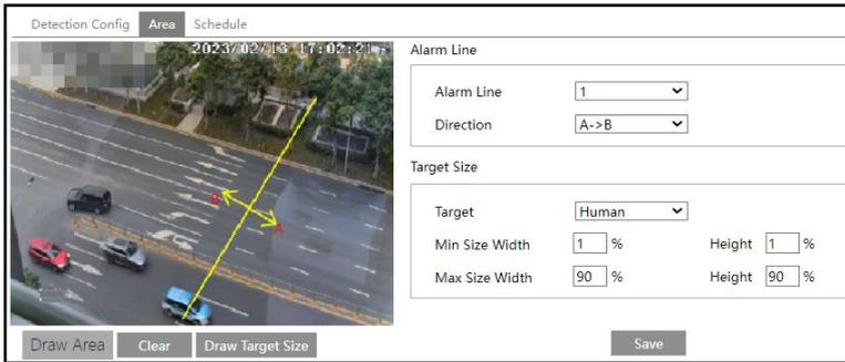
Set the alarm line number and direction. Up to 4 lines can be added. Multiple lines cannot be added simultaneously.
